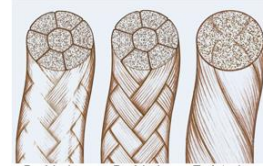
Braided Coated Braided Twisted Uncoated
